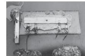
The first integrated circuit, a phase-shift oscillator, invented by Jack S. Kilby in 1958. (Courtesy of Texas Instruments.)
